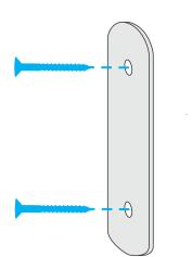
Attach the face by hooking the top and tightening the retaining screw at the bottom.
