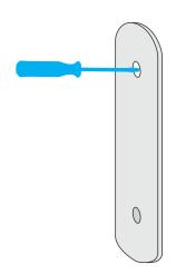
Attach back plate to the wall with the 2 provided screws.
